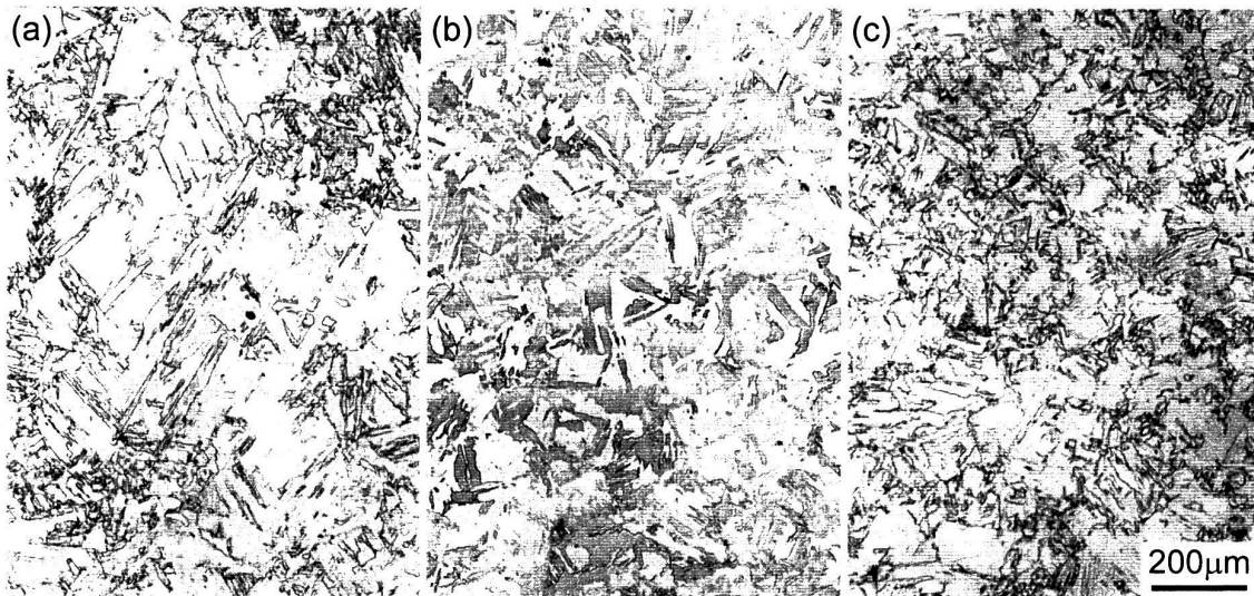
FIGURE 4. Optical micrographs of 8%Ni steel (a), 8%Ni-1%Cu steel (b) and 8%Ni-3%Cu steel (c). The steels were subjected to solution treatment at 1273 K for 30 min, then water-quenched and subzero treated at 77 K
